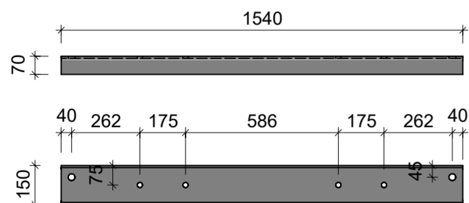
detail: 2400-108.ipt KGU 70 mm x 150 mm x 70 mm d=8 mm ( 1:20 ) met gtn Ø26/20
