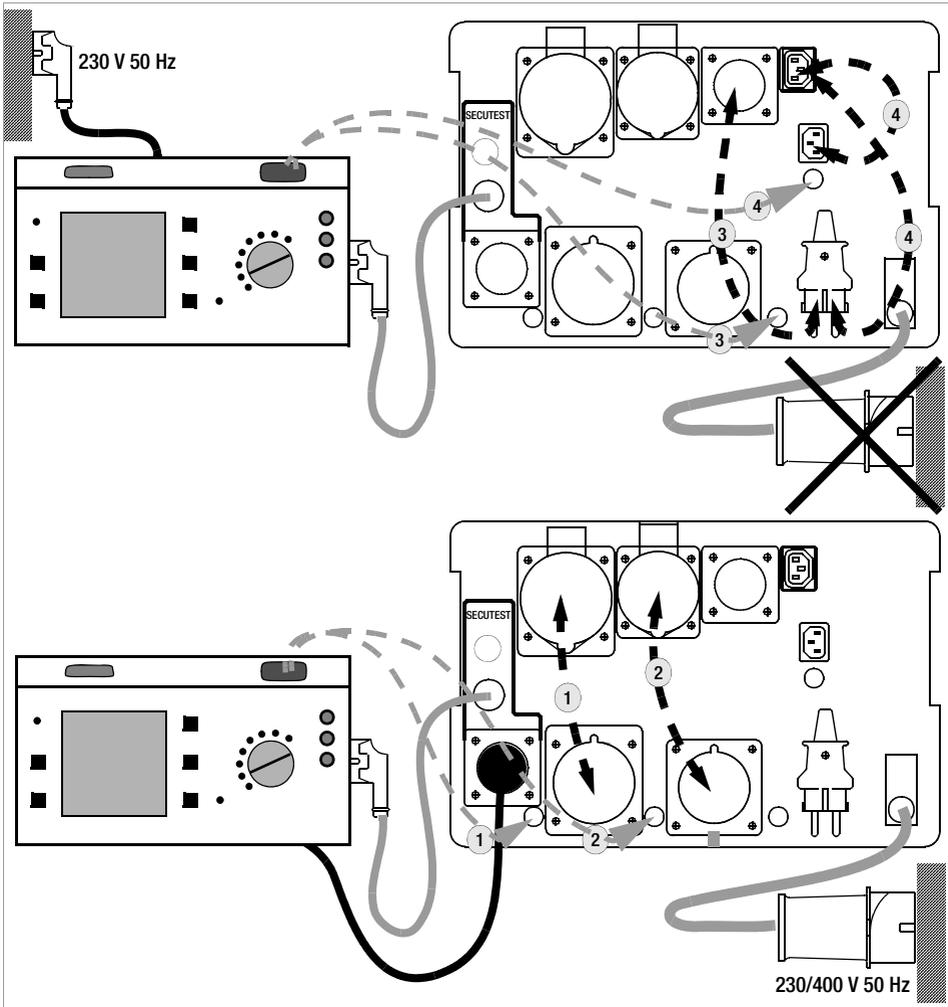
Figure 2 Connecting Single or 3-Phase Extension Cables to the AT3-III E with the SECUTEST...
