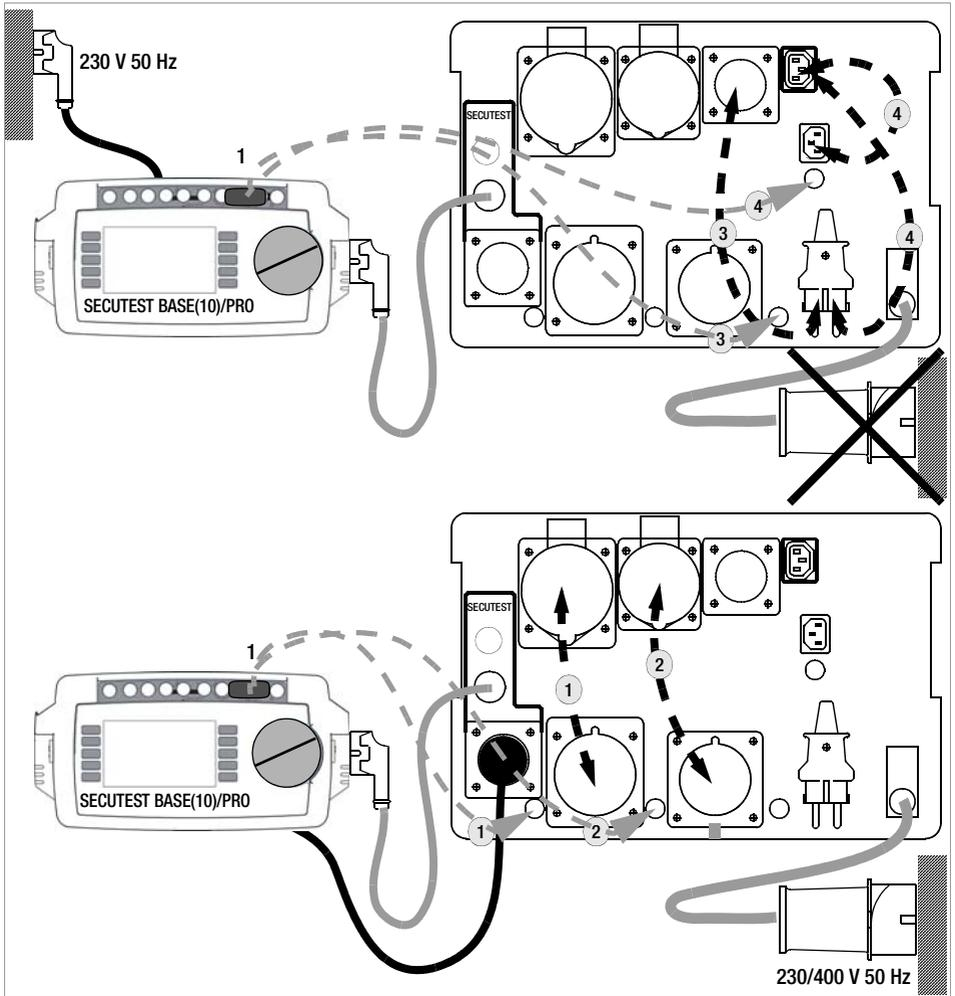
Figure 3 Connecting Single or 3-Phase Extension Cables to the AT3-III E with the SECUTEST BASE(10)/PRO
