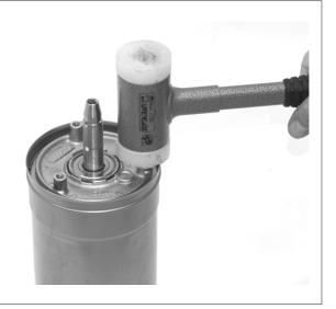
17. Fit the outer casing and the spring ring. Pull the shaft-rotor unit against the spring.
