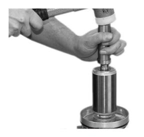
4. Fit new O-rings to the bearing housing.
