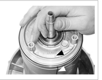
16. Gently hammer on the three bosses to get the shaft-rotor unit in place. Check that the spring groove is visible.
