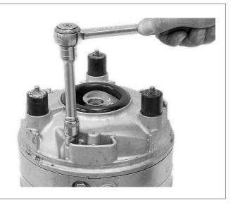
30. Using a 8 mm hexagon bit adaptor ( allen socket) with a 100 mm (4") extension, turn the adjustment screw clockwise until the impeller makes contact with the suction cover. Tighten it further 1/8 turn, 45°. This will ensure the correct clearance between the impeller and the suction cover in the next step.
