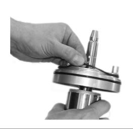
Fit a new O-ring to the stator housing unit.
