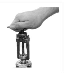
26. Press out the lower bearing with a press, or use the dismantling tool, (see page 5).
