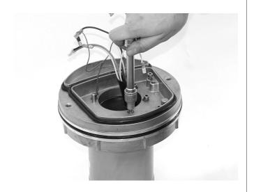
10. Mount the starter unit and connect the stator leads.
