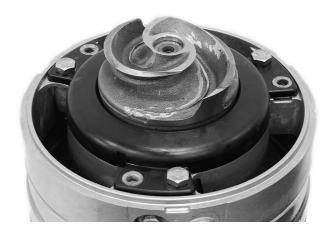
28. Before assembly, check that the impeller screw is clean and easy to screw into the shaft end (a). This to prevent the shaft to rotate with the impeller screw. Assemble the conical sleeve and the impeller onto the shaft.
