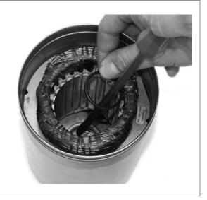
6. Fit two new O-rings to the ring and mount it to the stator housing.
