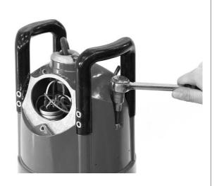
15. Place the pump upside down. Fit the rotor unit. The arrow mark on the bearing holder should point in the same angle as the drawn line on the stator housing.
