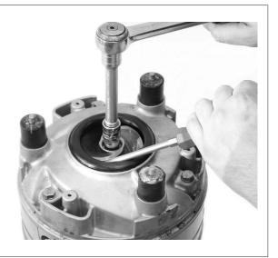
13. Disassemble the diffuser. Use a screwdriver or similar to seperate the diffuser from the intermediate piece.
