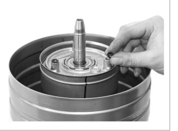
19. Fit two new greased O-rings on the intermediate piece.
