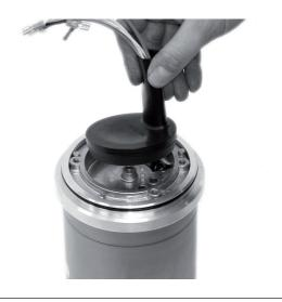
8. Make a line on the stator housing from the arrow mark on the upper bearing holder.
