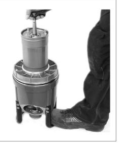
24. Press out the bearing housing with a press, or use the dismantling tool, (see page 5).
