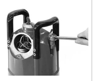
3. Disconnect the power and the ground cable leads.
