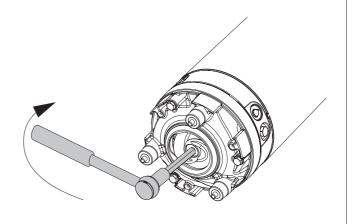
31. Lock the impeller with a screw driver or similar (L= min. 200 mm/7.9 inch), see fig., to prevent rotation of the impeller. Fit the washer and the greased impeller screw and tighten, torque to 22 Nm (16 lbf-ft).
