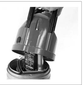
4. Remove the air valve if needed.
