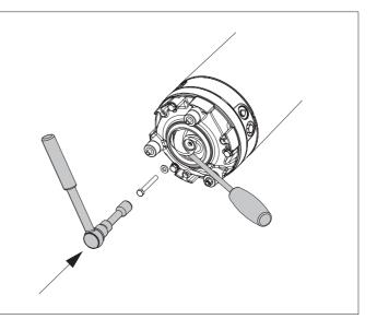
32. Mount the strainer and nuts, tightening torque 17 Nm (12.5 ft lb).
