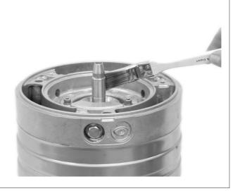
22. Fit a new mechanical seal unit (oiled).
