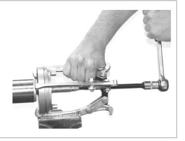
25. Use a standard puller to remove the upper ball bearing.
