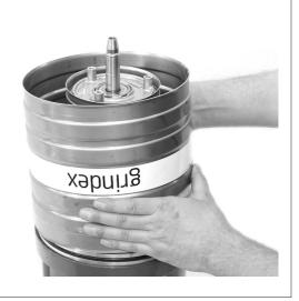
21. Gently hammer on the three bosses a few millimeters to expose the spring ring.
