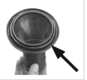
35. Asseble the connection flange on the discharge connection and tighten the connection flange to the cover.
