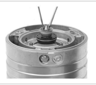
25. Assemble a new set of pressure equalizers.
