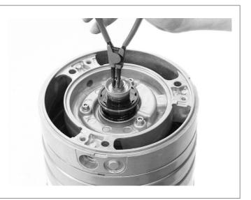
17. Remove the mechanical seal.
