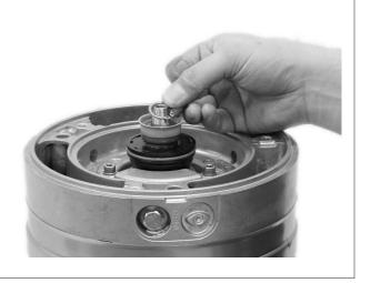
24. Press down the retaining ring by using two screwdrivers or a tube in suitable size. Control that the retaining ring enters its groove properly.
