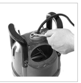
6. Disconnect the stator leads and remove the starter unit holder.
