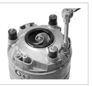
14. Using a 8 mm hexagon bit adaptor (allen socket) with a 100 mm (4") extension, turn the adjustment screw counter clockwise until the impeller breaks free from the shaft.
