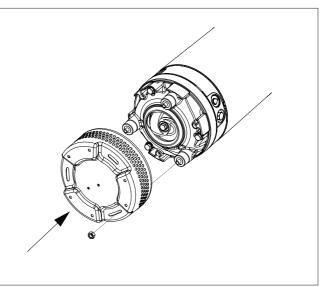
33. Put one of the oil screws **(a)** back and tighten it. Fill up with new oil.
