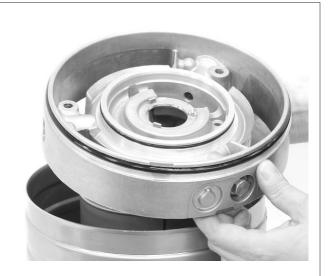
20. Fit the intermediate piece on the drive unit.
