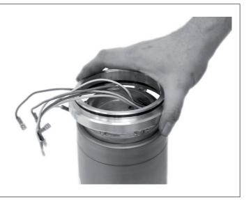
7. Pull the motor cables trough the protective casing.
