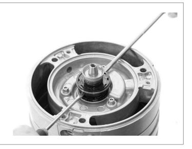
18. Remove the screws holding the intermedate piece.
