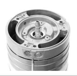
20. Remove the outer casing.
