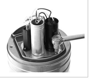
7. Remove the cover and the outer casing.
