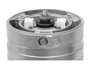
26. Fit a new greased O-ring and mount the seal housing cover.
