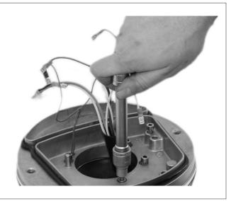
8. Remove the protective casing.
