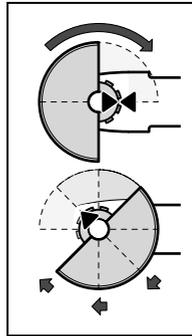
Place the protection guard **12** onto the spindle collar as shown in the illustration. The triangle marks on the protection guard must correspond with the respective marks on the gear case.
