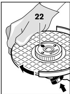
Lock the grinder spindle with the spindle lock button 2. To tighten the quick-clamping nut, firmly turn the grinding disc in clockwise direction.
