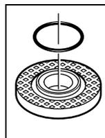
An O-ring (plastic part) is inserted in the mounting flange **8** around the centering collar. **If the O-ring is missing or is damaged, it must in all cases be replaced (article number 1 600 210 039) before the mounting flange 8 is mounted.**
