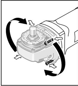
The machine head can be rotated with respect to the machine housing in 90° steps. In this manner, the On/Off switch can be brought into a more convenient position for special working situations, e.g., for cutting op-
