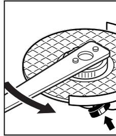
A properly attached, undamaged quick-clamping nut can be loosened by hand when turning the knurled ring in anti-clockwise direction. **Never loosen a tight quick-clamping nut with pliers. Always use the two-pin spanner.**
