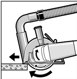
Switch on the machine and place the front part of the cutting guide on the workpiece. Slide the machine with moderate feed, adapted to the material to be worked.
